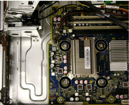
Figure 6-60 Removing the heat sink
